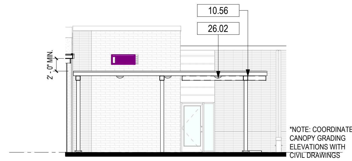
C4 GYM COVERED WALKWAYS - WEST ELEVATION 1/8" = 1'-0"
