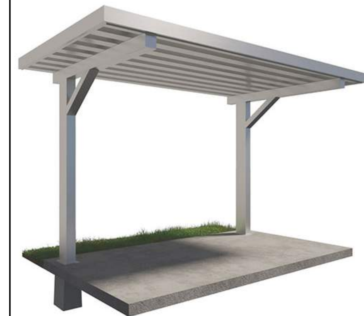
B - CANTELIVERED BENT WALKWAY
