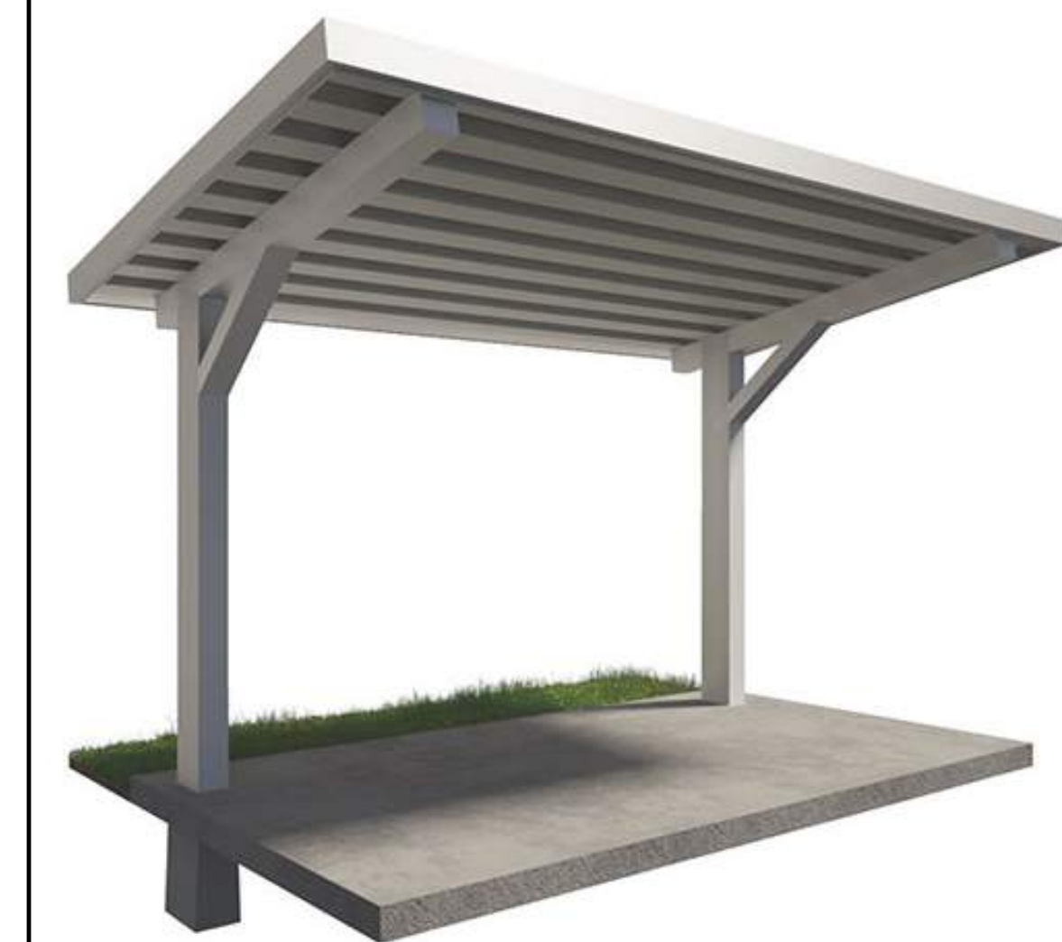
C - SLOPED CANTELIVERED BENT WALKWAY
